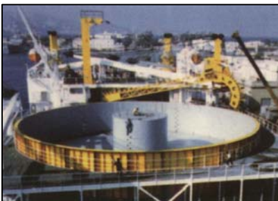
Tube umbilical being transferred from the manufacturing process into the storage carousel via the loading arm.
