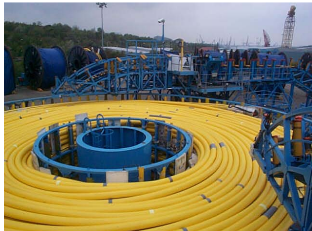
Fully loaded carousel showing additional wall diameter to suit product MBR.
