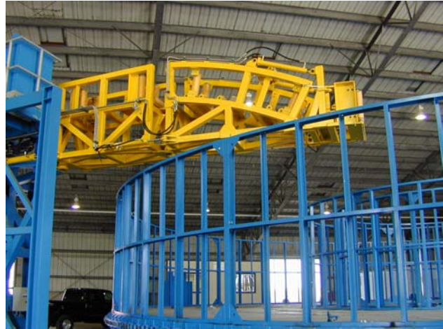
Carousel loading arm supported from a gantry tower. The arm is designed to protect the product minimum bend radius and can slew from outer to inner walls and articulate vertically to make loading and unloading 100% product friendly.
