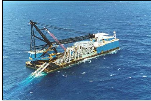
S-lay barge with storage reel, 550Te tension capacity and submerged stinger.
