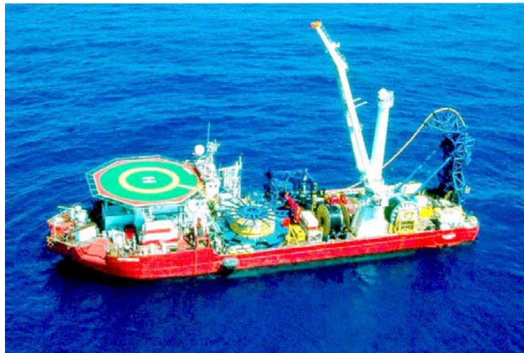
120Te capacity ramp with 1750Te horizontal reel
